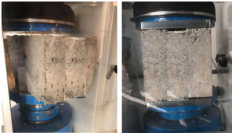
Figure 3: The circular machine tool (left) and the plates added above and below the block (right).
