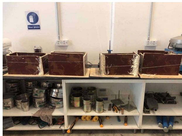
Figure 1: The forms used to create the samples on the right and the inside of a form before casting on the left.
